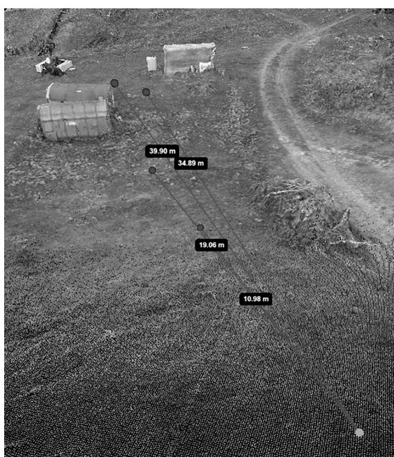
Fig. 6. Measuring distances using dense point cloud
