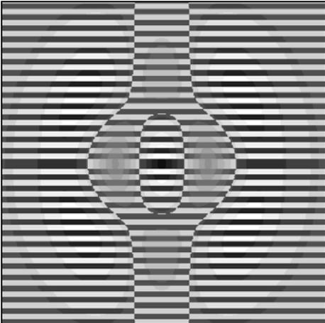
Fig. 5: Phase mask of manufactured MODAN (central part)
