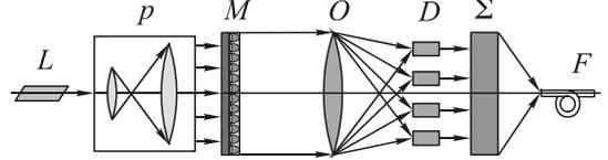
Fig. 16: General scheme of a multichannel waveguide telecommunication system. **L** - laser light source, **P** - collimator, **M** - MODAN, **O** - Fourier stage, **D** - set of modulators, **F** - ideal parabolic index fiber.
