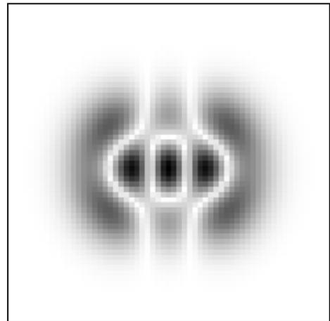
Fig. 4: Amplitude distribution in the cross-section of the invariant beam after propagation through a Fourier-stage (computer simulation)
