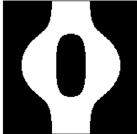
Fig. 3: Theoretical phase distribution in the cross-section of the invariant beam (black corresponding to phase 0, white - to  $\pi$ )
