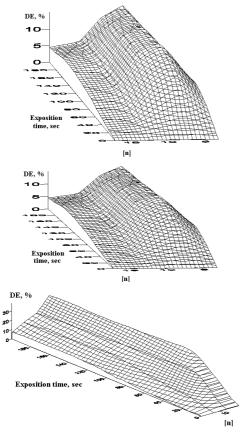
Fig. 2. The diffraction efficiency vs the time of exposure by the light of 10 mW/cm<sup>2</sup> for the SD DG layers with the gelatin concentrations:
