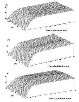
Fig. 1. The change of kinetics of the normalized optical rotation angle at 20C for SD DG layers with the gelatin concentration: a) 3%, b) 7%, c) 10%. [n] = glycerol concentration.
