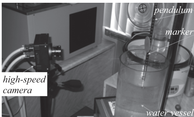
Fig. 6. Picture of the unit for investigation of damped oscillations of the physical pendulum
