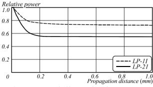
Fig. 3. Beam power in the fiber core depending on propagation distance for LP-11 (upper line) and LP-21 (lower line)
