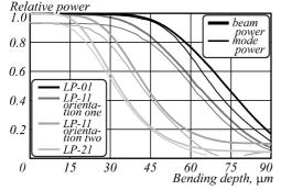
Fig. 9. Beam power in the fiber core depending on microbenging depth for LP-01 (the first from the top), two orientations of LP-11 (the second and the third from the top) and LP-21 (the first from the bottom). Thick lines represent full beam powers and thin lines represent mode powers
