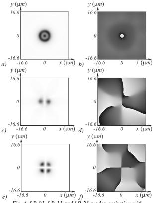
Fig. 4. LP-01, LP-11 and LP-21 modes excitation with Gaussian beam. Cross-section amplitude distributions (a), (c) and (e) and phase distributions (b), (d) and (f) are formed using no microrelief, and microreliefs shown in Fig. 1 (c) and (d), respectively
