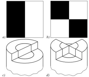
Fig. 1. LP-11 and LP-21 modes excitation. Phase functions (a) and (b) were implemented as microreliefs (c) and (d)
