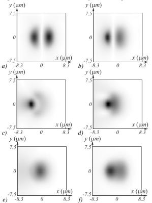
Fig. 8. Amplitude distribution in cross-section (orthogonal to the fiber axis) for the LP-11 mode in orientation two with bending depth of 74  $\mu$ m for different propagation distances: 0 mm (a), 0.2 mm (b), 0.4 mm (c), 0.6 mm (d), 0.8 mm (e) and 1 mm (f)
