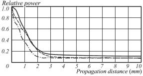
Fig. 5. Beam power in the fiber core depending on propagation distance forLP-01 (upper line), LP-11 (middle line) and LP-21 (lower line)
