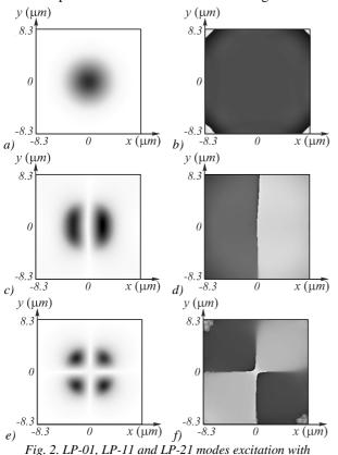
Gaussian beam. Cross-section amplitude distributions (a), (c) and (e) and phase distributions (b), (d) and (f) are formed using no microrelief, and microreliefs shown in Fig. 1 (c) and (d), respectively
