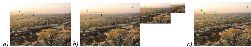
Fig. 18. The result of recognize circles in very complex conditions: (a) the original image; (b) a set of compressed images during processing; (c) the resulting image with recognized circles and unrecognized objects
