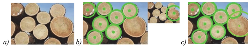
Fig. 16. The result of recognize circles for simple conditions: (a) the original image; (b) a set of compressed images during processing; (c) the resulting image with recognized circles
