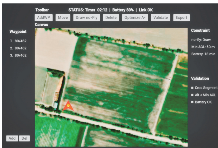
Fig. 1. Structure of widgets for agricultural UAV mission planning
