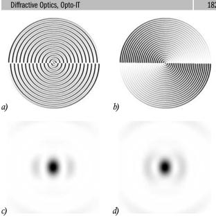
Fig. 1. The phase function of the DOE (a) forming the intensity distribution in the form of a single trap (b) in full correspondence to the standard, the phase function of the DOE (b) forming the intensity distribution in the form of the single trap (b) with incomplete correspondence to the standard
