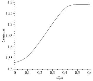
Fig. 6. Dependence of the image contrast C on the ratio  $d/p_0$  ( $\Delta n = 0.01$ ,  $d = 6 \mu m$ , c = 1.1%)
