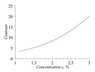
Fig. 2. Dependence of the image contrast C on the dye concentration c (d = 6  $\mu$ m, Dn = 0.2,  $\Phi_{\tau}$  = 900)
