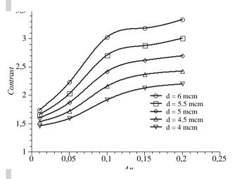
Fig. 1. Dependence of the image contrast C on anisotropy  $\Delta n$  of the refraction index (c =1,1 %,  $\Phi_{\tau}$  = 900)
