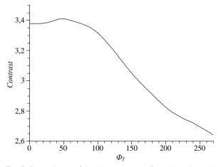
Fig. 3. Dependence of the image contrast C on the twist angle  $\Phi_{\tau}$  of LC structure (d = 6  $\mu$ m,  $\Delta$ n = 0.2, c = 1.1 %)
