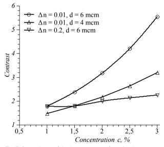
Fig. 7. Dependence of the image contrast C on the dye concentration c ( $\Delta n = 0.01$ , d = 6  $\mu m$ , d/ $\rho_0 = 0.5$ )
