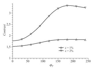
Fig. 5. Dependence of the image contrast C on the twist angle  $\Phi_{\tau}$  of LC structure ( $\Delta n = 0.01$ ,  $d = 6 \ \mu m$ )
