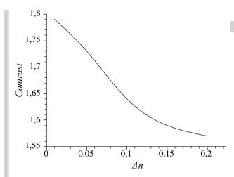
Fig. 8. Dependence of the image contrast C on anisotropy  $\Delta n$  of the refraction index (c =1.1 %,  $d/p_0$  = 0.5, d = 4  $\mu m$ )
