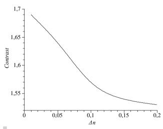
Fig. 4. Dependence of the image contrast C on anisotropy  $\Delta n$  of the LC transmittance index ( $\Phi_{\tau}$  = 900, d = 6  $\mu m$ , c = 1.1%)
